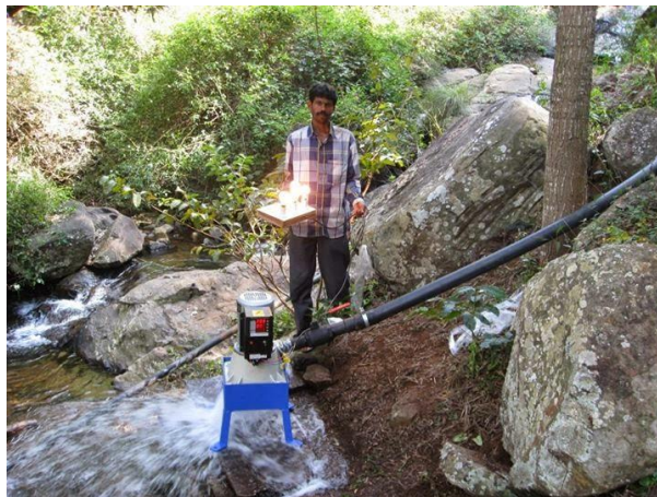
Figure 6: Pico hydro in operation
