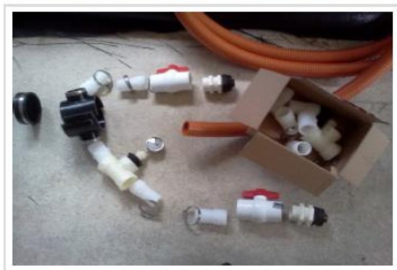
Figure 4: Pico hydro Piping Control elements (Source:
